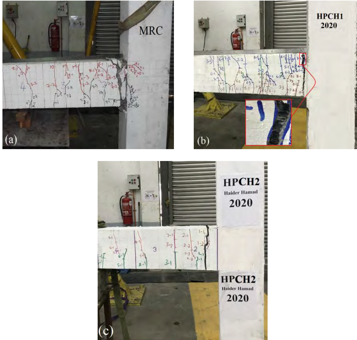
Fig. 4 Failure mode of the (a) MRC sample, (b) HPCH1 sample, and (c) HPCH2 sample.
