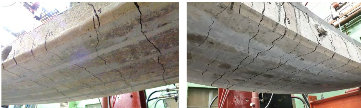
Fig. 4 Cracks at the bottom surface of the panels after executing experiments. Left figure is reference panel and right figure is panel with 30 mm UHPC.
