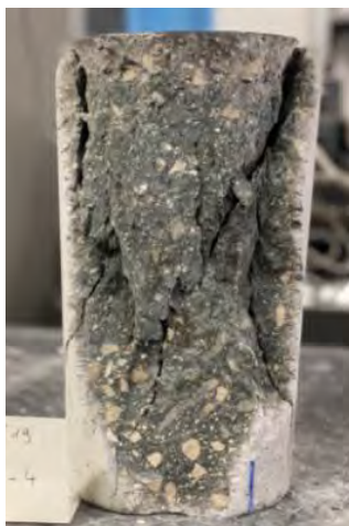
Fig. 4 Cylindrical specimen after failure after compressive strength tests (left) and stress-strain curves of GPC (right)
