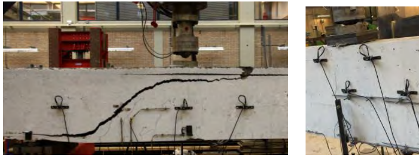
Fig. 1 Left: Beam RSB03A after shear failure. Right: Beam P804A1 after flexural failure.
