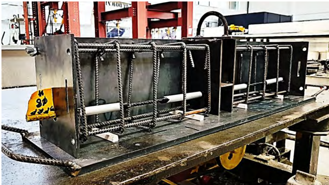
Fig. 3 Sample reinforcement during assembly in the mold
