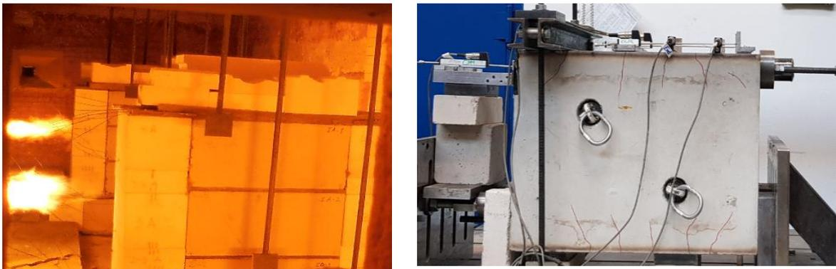
Fig. 4 a) beam-end specimens inside the furnace. b) pull-out test on beam-end specimen after fire
