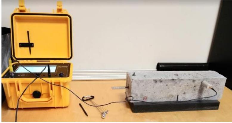
Fig.1 Stand for resonance frequency measurement of concrete prism samples.
