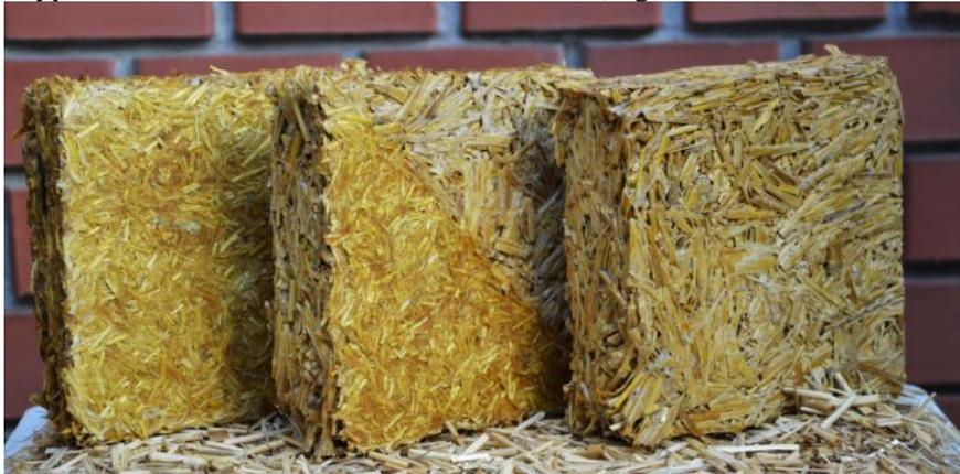
Fig. 1 Laboratory prototypes of the straw insulation
