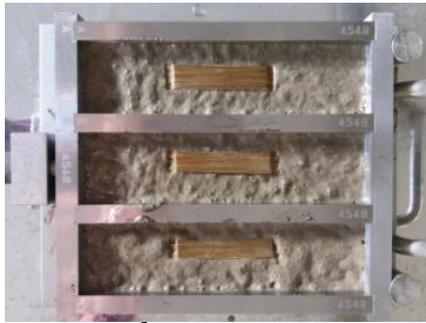
Fig. 1 A mould for three 40x40x160 mm<sup>3</sup> specimens – a demonstration of the steel fibres placement.
