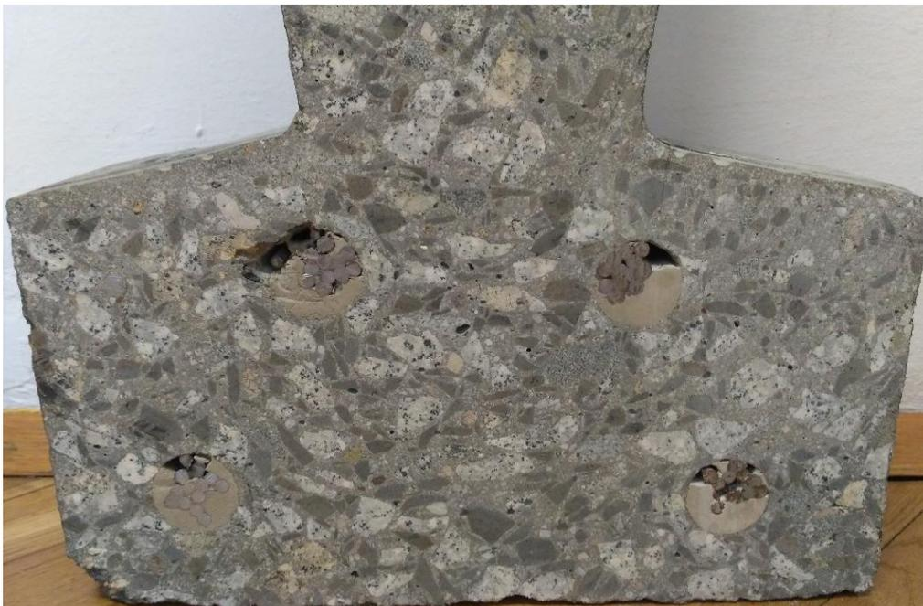
Fig. 6 Unproperly filled lower cable ducts on cut out cross-section of the tested beam.
