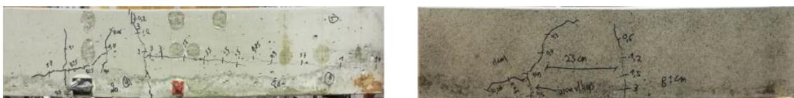
Fig. 5 Picture of cracks developed in the case of 5R1 (left) and 5R2 (right).
